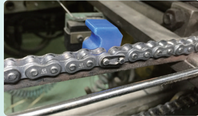
Replaced to TLH Roller chain - After 0 month
