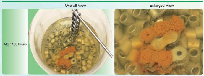
The solution became cloudy due to corrosion on the wholly immersed chain. No corrosion was observed on the hung chain.
