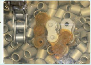
On the wholly immersed chain, corrosion started at the portions with a large contact area with the stainless steel parts. No corrosion was observed on the hung chain.
