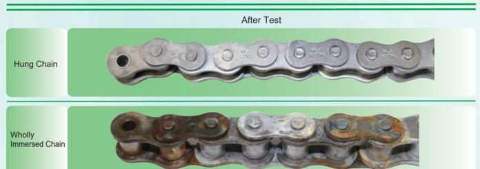
In the wholly immersed chain, electric current flew through the portions with a large contact area with the stainless steel parts, causing the TLH chain, which has excellent corrosion resistance, to corrode quickly.
