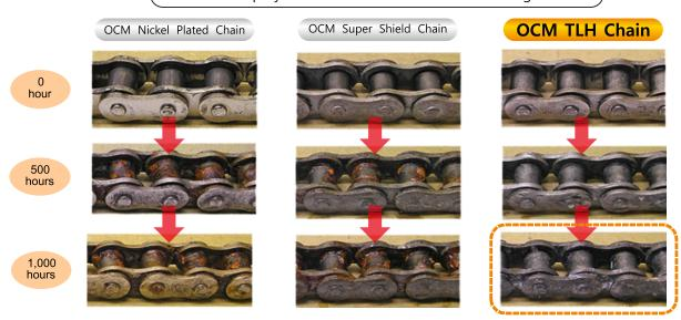
Interacting with Strong adhesion and Self-repairing makes the high anti-corrosion chain. After conducting 1,000 hours Salt Water-Spray test with the chain continuously running, no red rust was formed on the surface.
