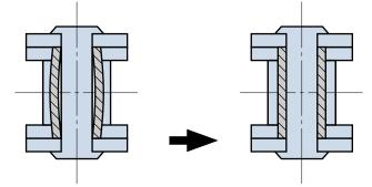
The advantage of solid bush, cylindrical roundness, making a large bearing area and oil port as an oil reservoir, improves the chain wear resistance and minimize an initial chain elongation.
