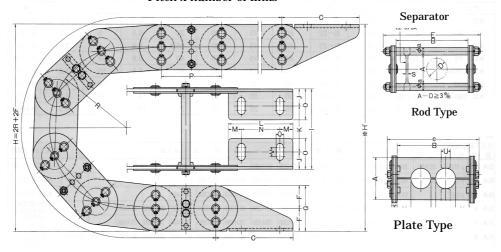
The minimum distance between holes of supporter should be 4mm.
